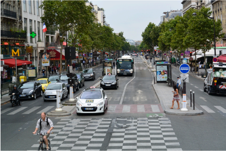
Boulevard du Montparnasse in Paris: example of a center-running-protected bus lane
